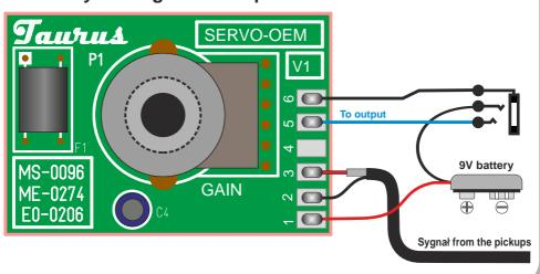
2. Option with SERVO ON/OFF switch. In this configuration two work modes are available: active mode (SERVO ON) and true bypass (SERVO OFF).
